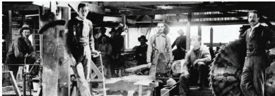
Above: Inside the Burrows Mill at Grandview. Powered by a 500 horsepower single-cylinder steam engine and driven by six horizontal tube boilers, each generating 125 pound per square inch (psi), the two circular saws squared and sawed the logs. All the belts and machinery were housed below the sawing floor, an innovation that Burrows introduced to Manitoba.
